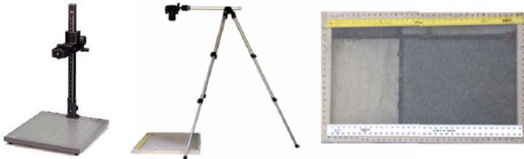
Figure 5. Equipment setup for capturing digital images of fish for morphometrics analysis: frontal view of Kaiser Repro table, side view of horizontal tripod with camera, and mesh cradle with ruler for displaying fish.
