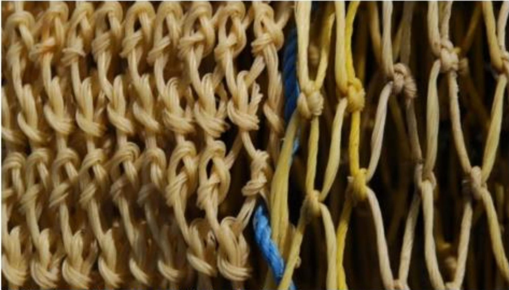
. Hand-woven (left) and machine-woven (right) codends.
