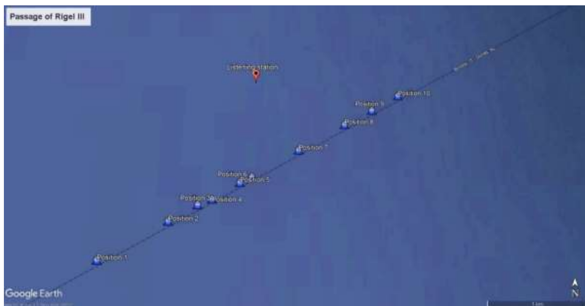
Figure 10. Figure reporting listening station and the progressive positions of the ferry Rigel III. For each position we measured the distance from the ferry to the boat, i.e. the listening station.
