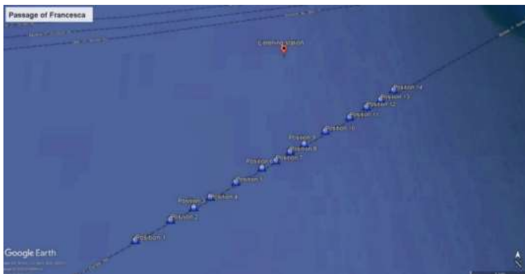
Figure 11. Figure reporting listening station and the progressive positions of the ferry AF Francesca. For each position we measured the distance from the ferry to the boat, i.e. the listening station.
