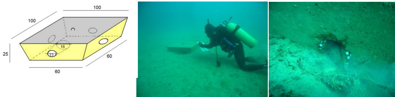
Fig. 11 – Turkey: production artificial reef units for octopus (courtesy of A. Lök).
