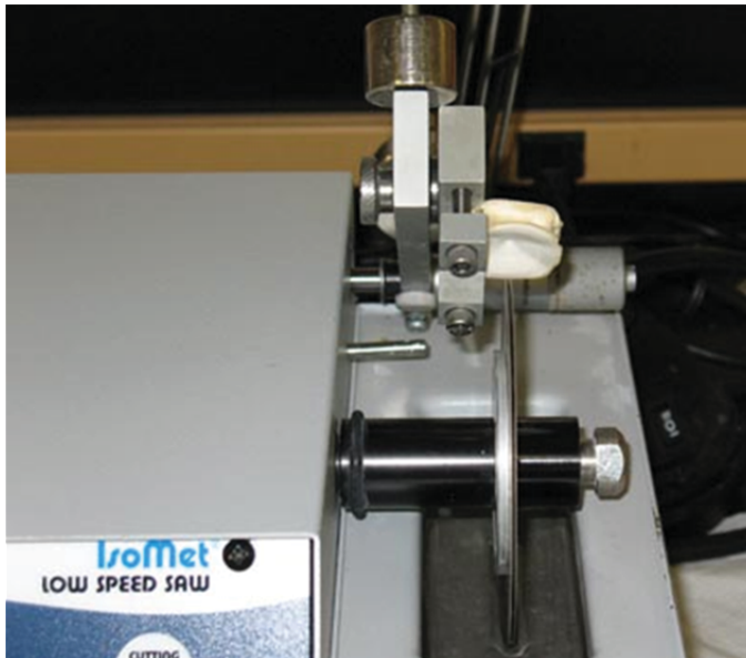
Figure 3. Preparing a section of a vertebra with an Isomet saw.
